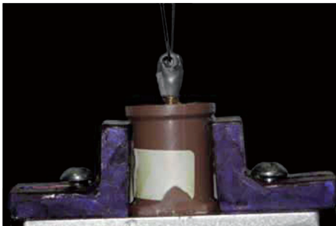
3 Specimen positioned for bond strength testing.
